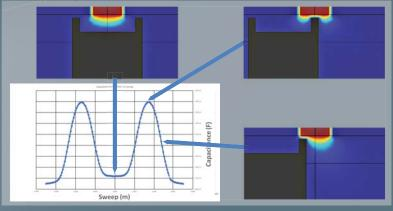
FEM capacitance calculation of blade passing in front of a sensor
