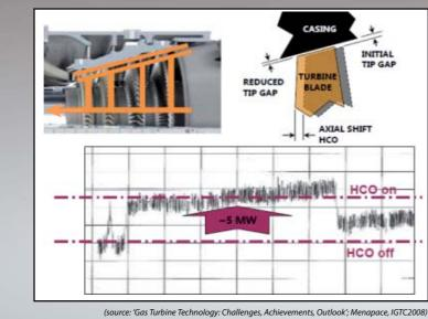
Blade Health Monitoring (BHM) is performed by mean of Real-time Blade Tip Clearance (BTC) and Blade Tip Timing (BTT) instrumentation based on non-invasive Capacitive technology.
